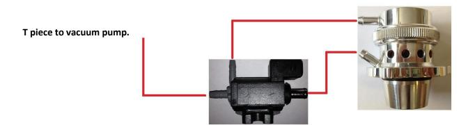
7. Take the solenoid and large cable tie provided and secure it to the large wiring loom next to the airbox vacuum pipe. Take the wiring loom supplied in the kit and connect it to the solenoid and the other end to the loom which was attached to the OE valve.
