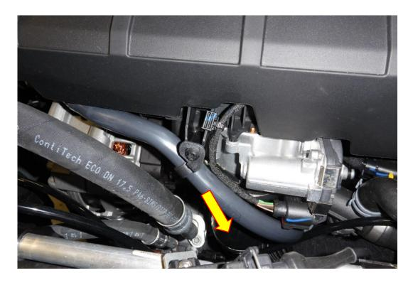
3. On the OE valve push back the red retaining clip to allow you to remove the wiring loom. Remove the three T25 Torx fasteners attaching the OE valve to the boost pipe, the OE valve will now come away.
