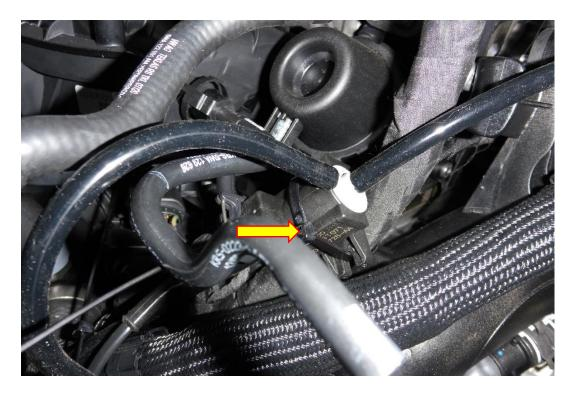
8. The vacuum source in the engine bay is next to where the solenoid has been fitted. Pull the vacuum pipe away from the plastic joiner.
