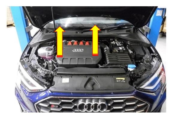
2. With the engine cover removed locate the original diverter valve. This is located on the boost pipe at the lower front of the engine.
