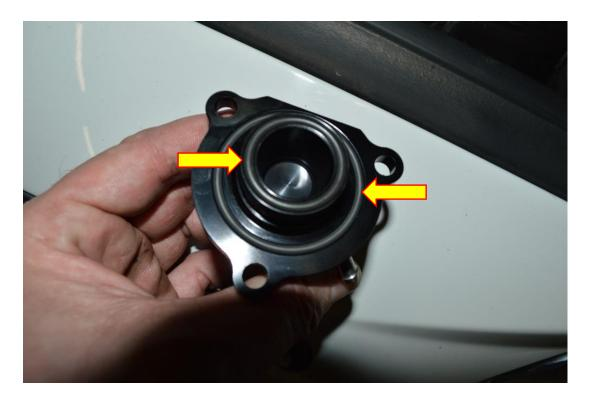
5. Take the Forge Motorsport valve and mount it into position where the OE valve used to be. Use the original T25 Torx fasteners to secure it in place.
