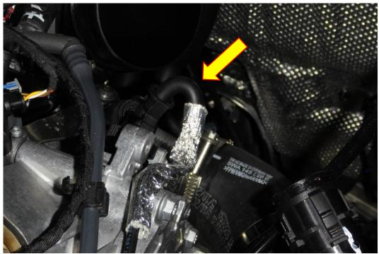
9. Using the supplied brass T piece and silicone pipe attach it to the vacuum pipe removed in the previous step just like it is in the picture below. Use the provided cable ties to secure the hose as shown with the arrows in the picture below.
